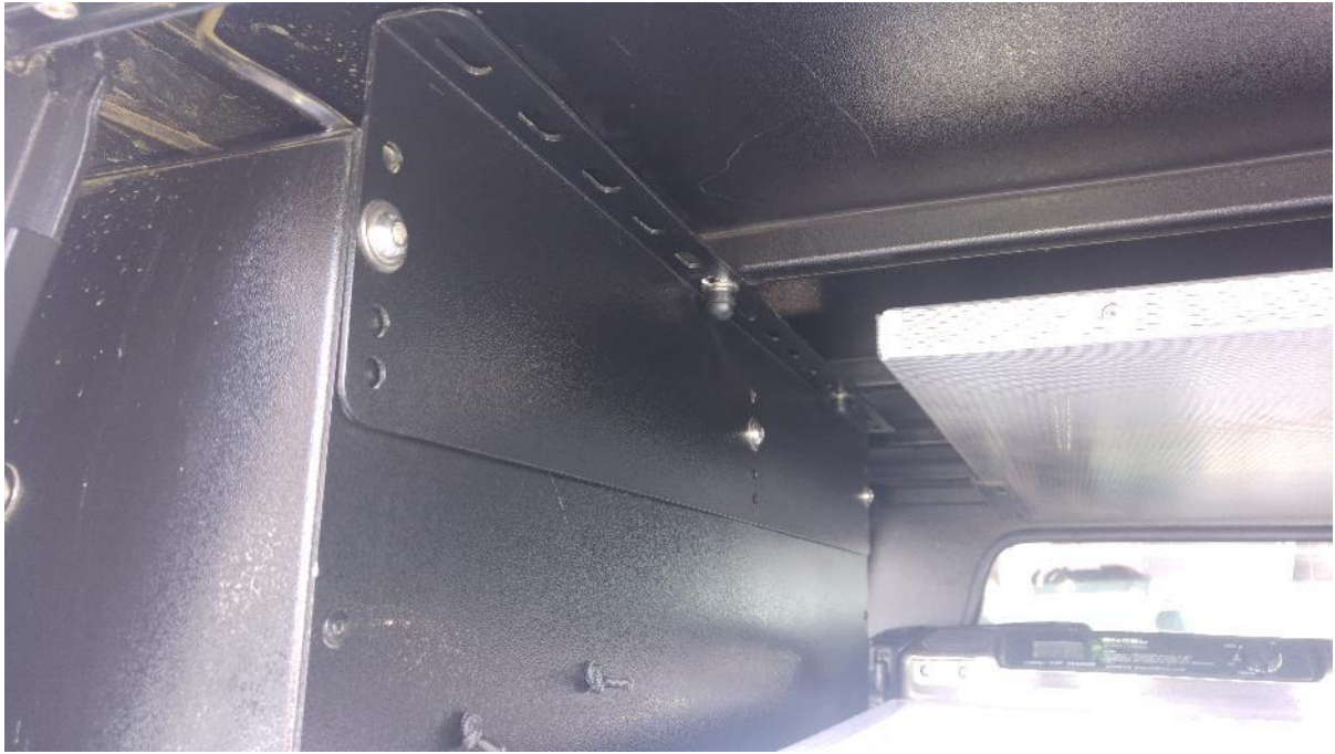
Photo of Assembled top bracket
