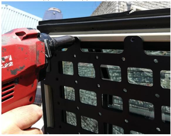
$\underline{\text{Step 6:}}$  Once all the rivets are in place the small molle plate should look like the one in the image below.
