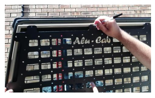
$\underline{\text{Step 6:}}$  Double check hole positioning and drill out the holes with a 5mm drill bit.
