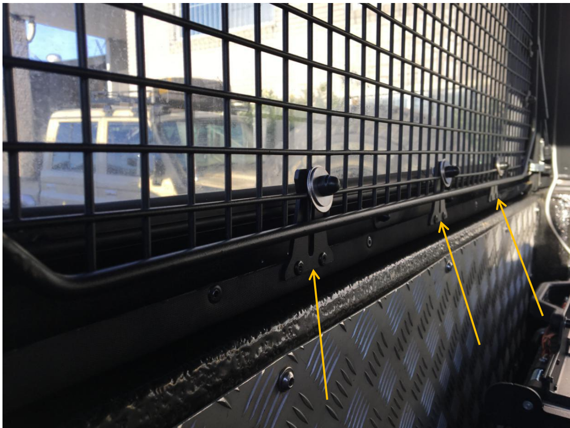
Figure 7: Three (3) equally spaced Bottom Vertical Mount Brackets riveted in place.
