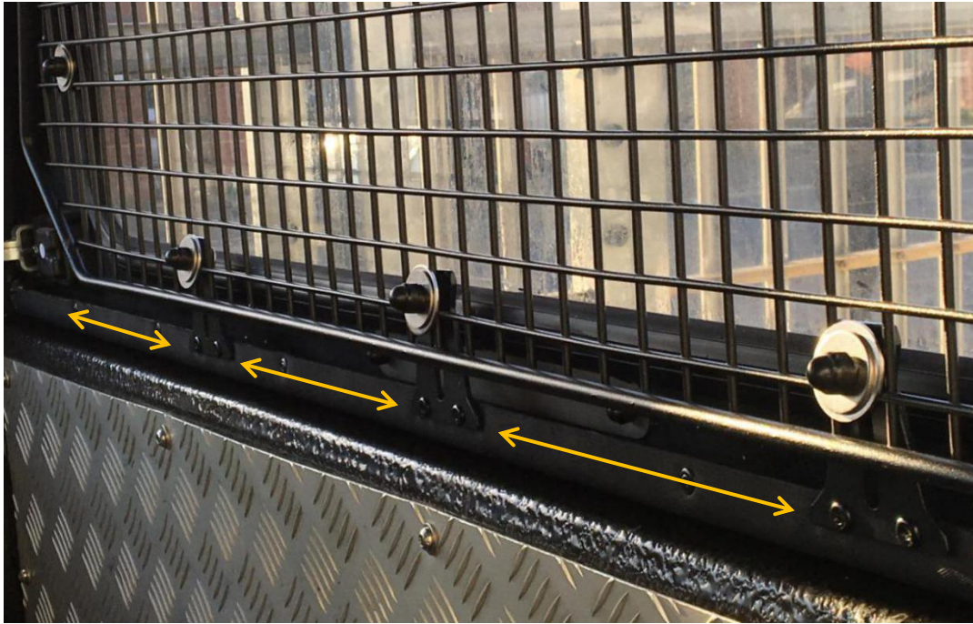
Figure 2: Measure and mark the equal spacing for the Vertical Mounts, with the center Vertical Mount located in line with the center of the Canopy Window.
