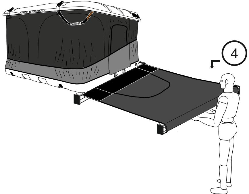
EN Unwrap the strips fixing the awning and unroll it. Remove both telescopic legs and place them on the ground. Lock them at the desired height, turning them in the direction as shown. Repeat the same operation with the horizontal tubes, fitting them in their assign locations and lock them by giving the correct tension to the awning.
